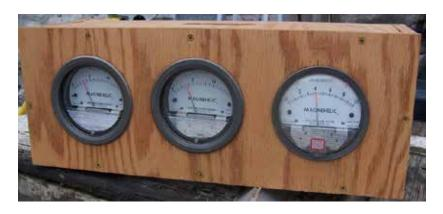
My gauge kit is home made, but effective. Two of the gauges read vacuum from 0-15 inches Hg. The other reads from 0-10. One verițes the others. I can disconnect the 0-10 gauge for elevated pressures.
