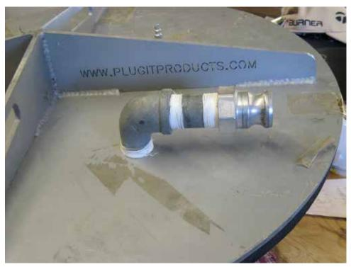
I have plumbed the top of the plate to receive the Cam-lock Ttting on the end of the twenty foot hose. At top is a quick connect which I connect to my gauges by a 25 ft air hose. I stand away from tanks that are being tested at high pressures. Testing at 4 inches Hg for water tightness is not usually a danger, but I have imploded concrete tanks at 10 inches Hg. Mid-seam concrete tanks usually stand 13 inches Hg. topseam tanks break at 8-10
