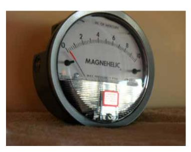
Gauges with a large face are easy to read. This one reads vacuum pressures from 0-10 inches Hg. It is easy to read small increments, like 5.1 inches Hg.
