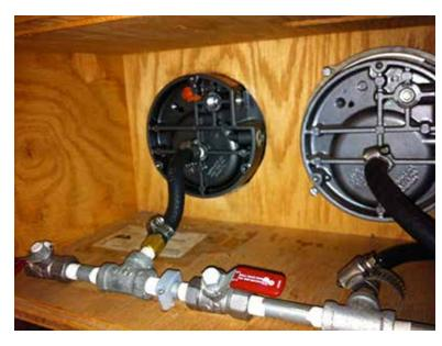
Inside my gauge kit I have plumbed the three gauges in series. By turning a valve, I can remove the 0-10 gauge from the series.
