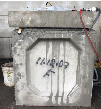
Ready for testing. The label indicates that this inlet box was made on November 12, 2007 with structural fiber reinforcement instead of steel.
