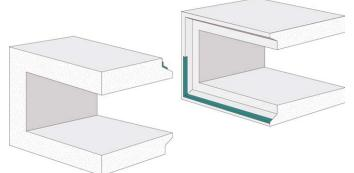
Sealant placed "outside will show when you look int the joint from outside the structure. Note that the ConSeal is placed on the leading edge of the bell and the back shoulder of the spigot.
