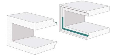
Sealant placed "inside" will show when you look down into the joints from the inside of the pipe or culvert. For a continous gasket this is where to put ithe butyl.
