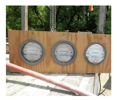
At 12.5 inches of Hg on the gauges, the tanks passes the requirements for H-20 loading. Nine pounds of Macrofiber per yard of concrete was used as the primary reinforcement in the sidewalls of the tank. The floor and roof are reinforced as directed by engineer's design. There is no steel in any of the sidewalls.
