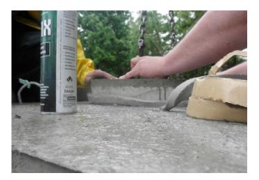
During the test, the manhole plug was sucked down into the opening. The gray CS-367 prevents leaks, while allowing easy disassembly. JEPCO SALES, LLC provided the test equipment. One end of the tank was sealed with CS-367 while the other end provided access to the tank for the equipment. Because the 24 inch openings are tapered, the 26 inch diameter test plate would not cover the opening. Plywood with CS-367 under it, and with an opening cut in it helped seal the opening
