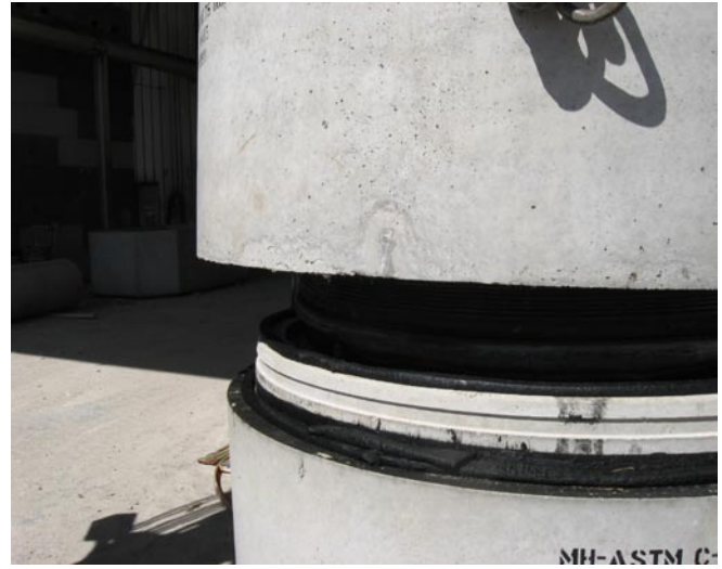
Ready to test with two strips of 7/8 size CS-102
