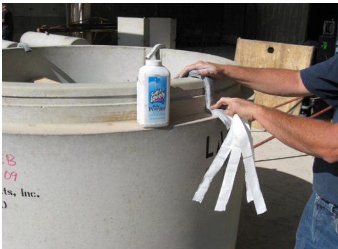
Talcum powder prevents adhesion during bite-wing
