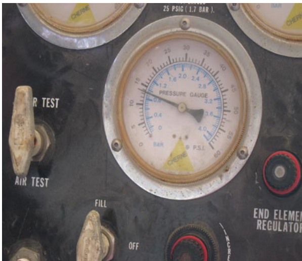
13.5 psi held watertight for 10 minutes
