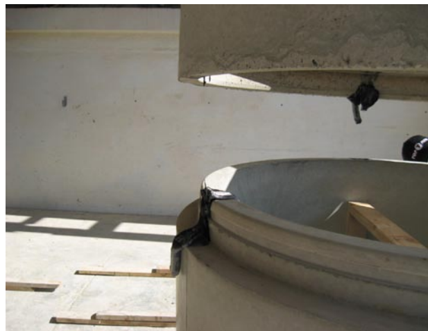
Crushed CS-102 reveals internal fit
