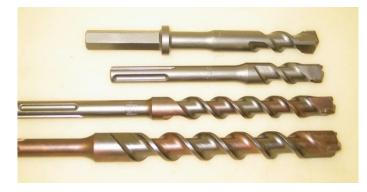
DRILL BITS: SDS MAX &WACKER HEX "Shorties" in either format (top two on left) are specially made to drill I" inch diameter holes in tight places. Great for step holes in manholes. Standard 1" inch bit is three times as long. Each bit has Quad-Carbide tips for durable, fast drilling
